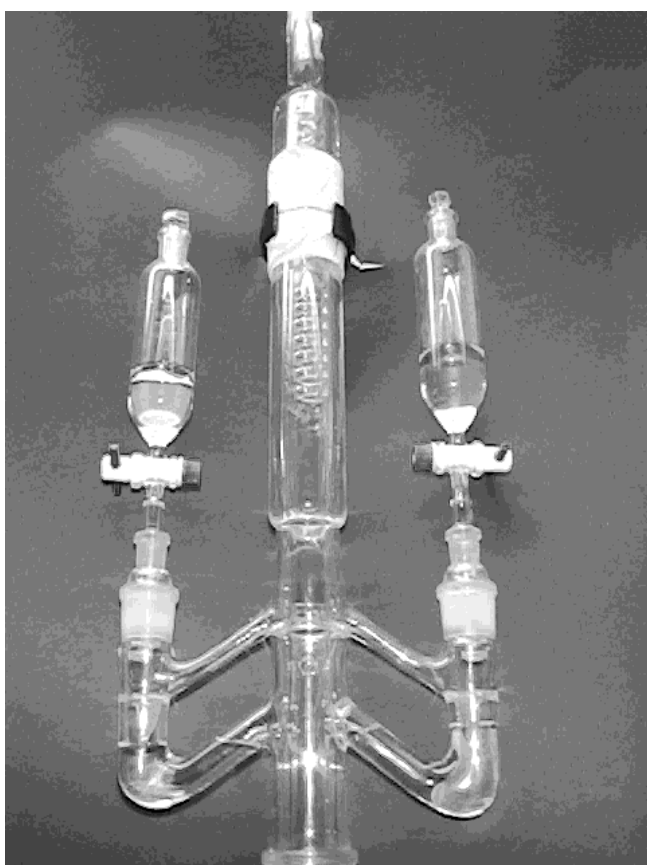
Fig. 1 Photo of the two component high dilution principle (2-C-HD) apparatus designed by Professor Vögtle and marketed [7] by Normag Labor- und Verfahrenstechnik GmbH (Hofheim, Germany) used in this work.
